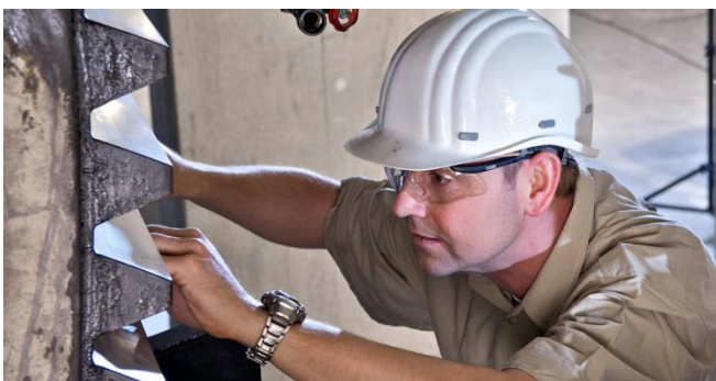
Checking the "static contact pattern" of large tooth gearing
