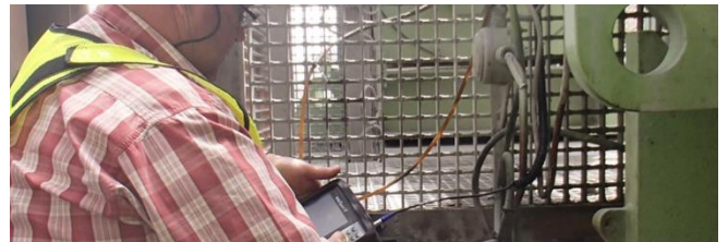
Measurements at planetary gear units with the vibration measuring device
